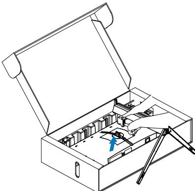
3. Press the button to remove the rear pillar cover
